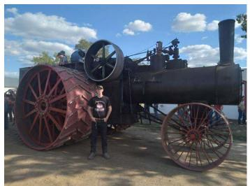
This tractor may only produce 150 horsepower but it has pulled 50 bottom plows at the same time.
